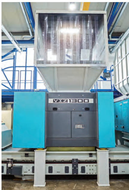
Vecoplan’s VIZ shredder can be equipped with either with a high-torque, quick-start drive or a frequency controlled, belt-type direct drive.
