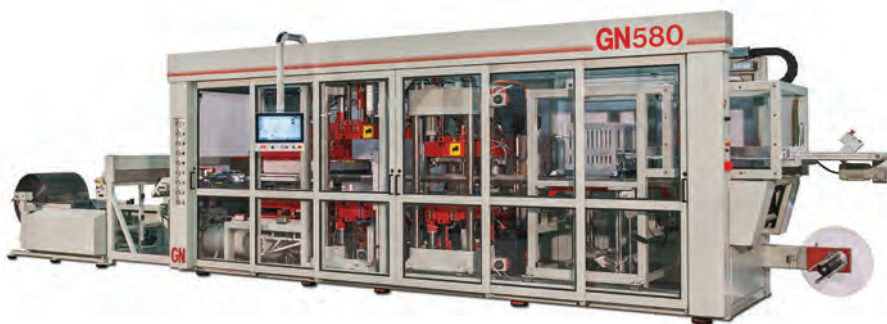
GN Thermoforming’s new form/cut/stack GN580 thermoformer.
