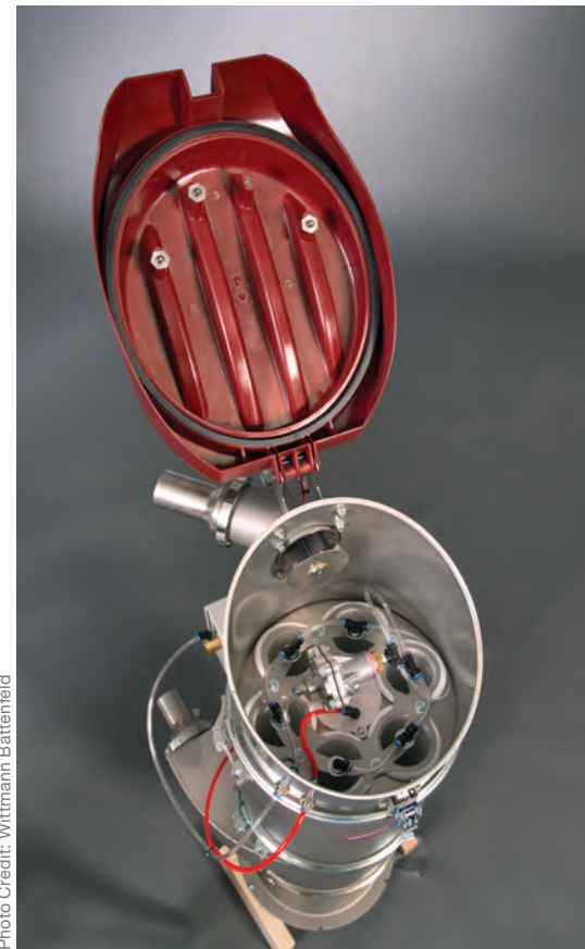
Wittmann Battenfeld’s PMX series powder loaders have a blowback system designed to extend the operational life of the filter media.
